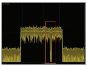
Figure 1b. Identification of a signal dropout with Real-Time Power Processing  $^{\mathtt{M}}$ .
